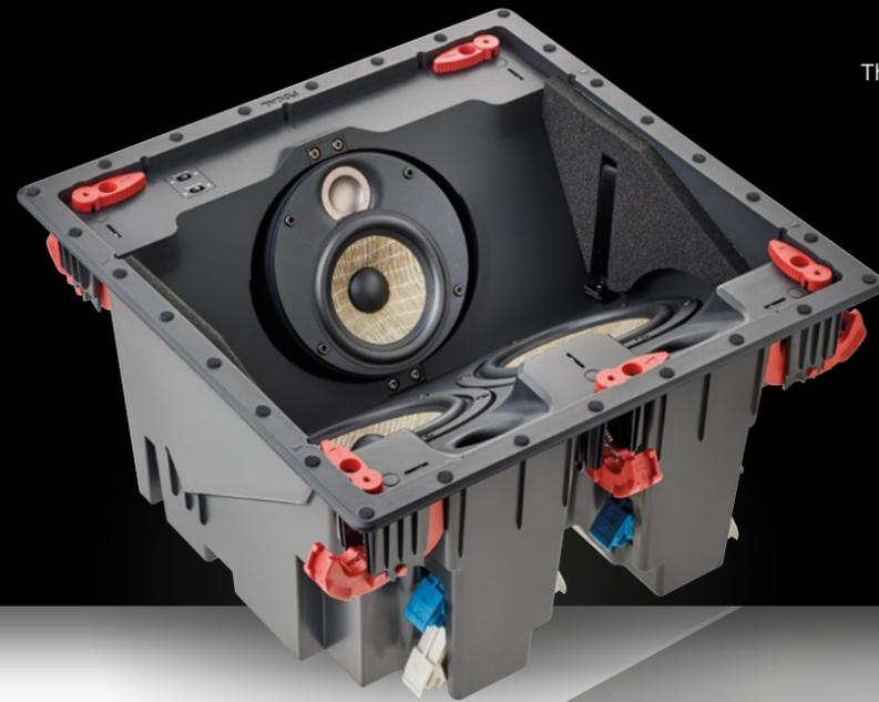
The 300 ICLCR5 is equipped with a left/centre/right channel selector to mechanically direct the sound towards the listening point, making it perfect for Home Cinemas. For in-ceiling loudspeakers, the dedicated 300 ICLCR5 is equipped with an adjustable tweeter housing for directing sound towards the listening point with precision. The tweeter level is also adjustable so that it can be set according to the room's acoustics, and the upper midrange can also be adjusted.
