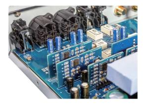
The phono input has a variety of settings for input resistors and capacitors to match different MM cartridges. PRA-9X phono amplifier is a 2-stage RIAA amplifier that utilises NJR MUSES8820 audio quality op-amp to provide an accurate RIAA curve and low distortion at high amplification and performance.
