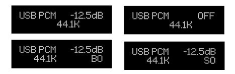
"BO" means "balanced only" and "SO" means "single-ended only".
