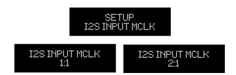
"1:1" means that the master clock is left unchanged. This is indicated when the master clock frequency is below 27MHz. "2:1" means that the input master clock frequency is halved. This is mandatory when the input master clock is 45.1584MHz or 49.152MHz.
