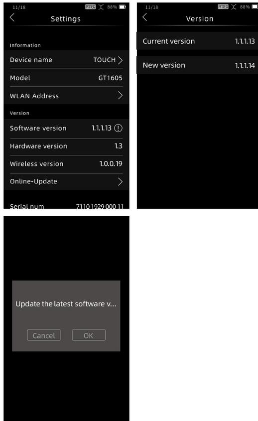
After a successful update, the player will automatically shut down. Upon powering on again, you can check the latest software version number in "Settings > Software Version."
