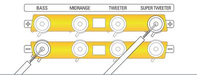
For optimum sound quality, connect the cable from the power amplifier to the terminals shown.
