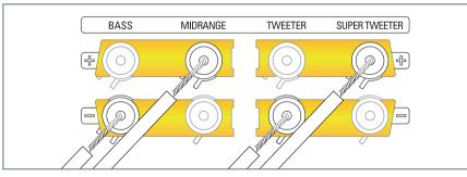
For optimum sound quality, connect the cables from the power amplifier(s) to the terminals shown.
