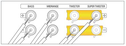
For optimum sound quality, connect the cables from the power amplifier(s) to the terminals shown.
