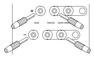
For optimum sound quality, connect the cables from the power amplifier(s) to the terminals shown.
