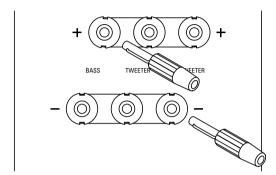
For optimum sound quality, connect the cable from the power amplifier to the terminals shown.
