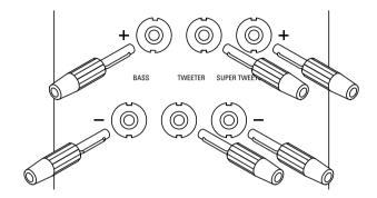
For optimum sound quality, connect the cables from the power amplifier(s) to the terminals shown.
