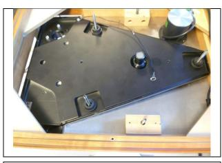
Carefully lower the sub-chassis section, ensuring that the LP12 suspension bolts pass through the grommets on the KORE.
