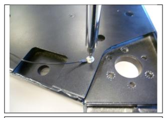
Using a T10 Torx driver, screw the earthing wire loop and washer onto the KORE with the supplied M3 x 6 Torx screw.
