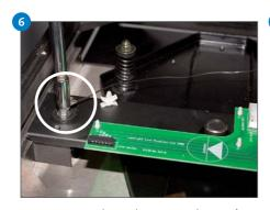
Use an 8 mm socket tool to remove the nuts from the wiring strap.
