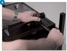
Fit the appropriate guard to the stylus.
