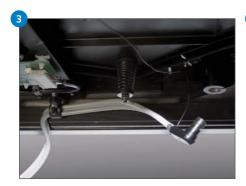
Loosen the grub screw at the base of the arm collar. Disconnect the arm cable from the underside of the tonearm.
