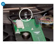
Clamp the power supply cable to the wiring strap. Ensure that there is no tension in the cable between the clamp and the connector but also ensure there is not too much slack. The cable shown is correctly adjusted.
