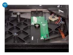
Reinsert the wiring strap. Ensure it is correctly oriented – the switch connector should be at the front of the LP12 and the power and motor connectors at the back.
