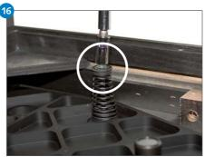
Carefully lower the sub-chassis section, ensuring that the LP12 suspension bolts pass through the grommets on the KEEL.
