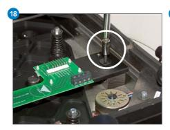
Refit a large washer and nut to each of the wiring strap bolts and tighten.
