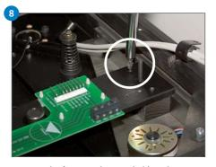
Remove the four wood screws holding the strap to the plinth (two at each end).
