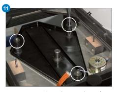
Using an 8 mm socket tool, remove the nut from each of the three suspension springs.
