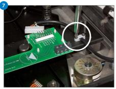
Remove the two screws holding the cable clamp.
