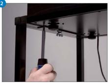
Remove all the screws holding the base board in place. Support the base as you do this.
