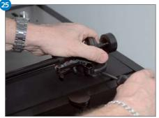
Refit the tonearm and tighten the arm collar bolt assembly.
