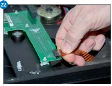
Reconnect all cables to the circuit board. If the flexible foil type of switch connector is fitted, ensure the silver side is facing upwards as shown.
