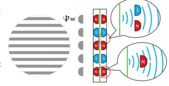
Degradation of sound quality in a conventional planar magnetic headphone is caused by the magnets getting in the way of the sound wave.
