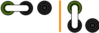
Figure 5. Wall socket earth applied
