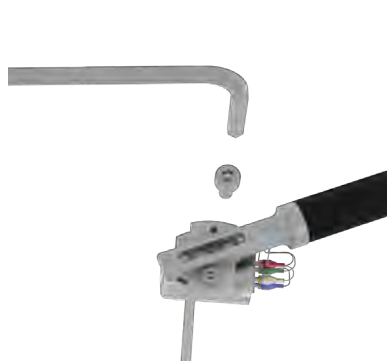
Pic. 8: Mounting the cartridge
