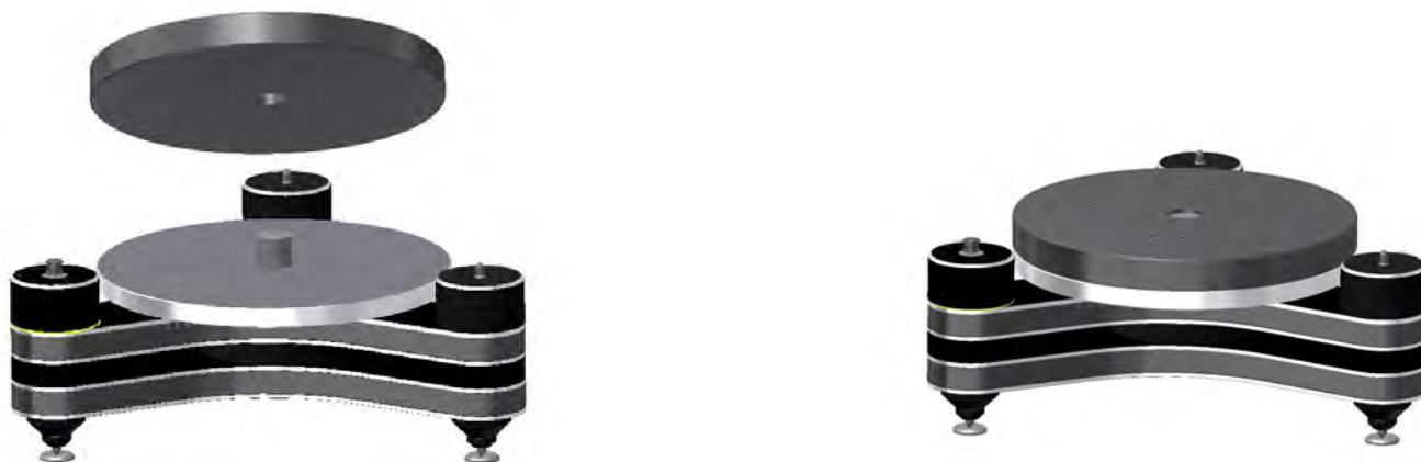
Pic. 9: Placing the drive unit platter onto the bearing
