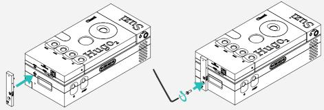
The USB Multiplexer offers both USB-B (data only) plus USB-C (data and charging) connections to the Hugo 2 DAC. Both connections can be made simultaneously and the Hugo 2 will auto-detect the signal for playback providing USB is selected as an input via the Hugo 2; see the Hugo 2 manual for operation information.
