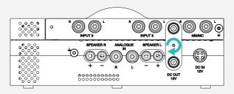
The respective power cables/supplies can now be attached and with all connections made as per section 4 Connections and Controls and the respective Suzi Pre manual, power to the units can be switched on, and the Suzi power amp power button depressed, to make the units ready for playback.
