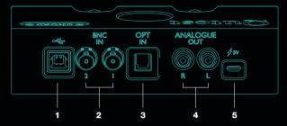
USB Type-B input: 32-bit 768kHz PCM/up to DSD 512 2x BNC coaxial input - 24-bit/384kHz/Dual-data mode capable to 768kHz Optical input: 24-bit/192kHz DSD 64 RCA analogue outputs (Left and Right) Micro USB power supply input - 5V 1-amp minimum
