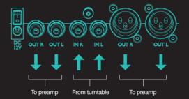
Once Huei is connected, do not switch your preamp/amplifier 'on' until the volume is at its lowest setting. Next, turn Huei 'on' and select the appropriate settings for your cartridge as explained below. With the settings correct, select the lowest gain setting on Huei (white), before turning connected equipment 'on'. Next, select the appropriate input on your preamplifier, begin playing the source and gradually increase the gain/volume to a comfortable level.
