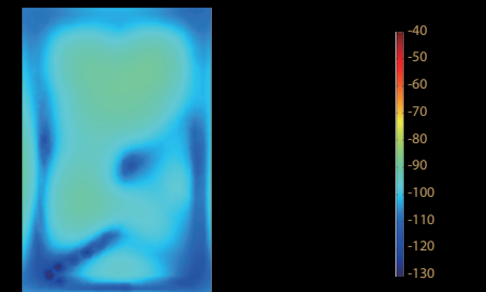
ABOVE: Laser vibrometre measurement of a cabinet at 400Hz after optimisation
