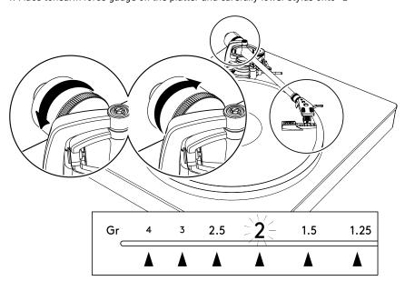
Adjusting the counterweight ensures the pressure the stylus applies to the record is correct. Too much pressure can cause distortion and lost information as well as wear to your records. Too little pressure and the stylus will jump and potentially damage your records.
