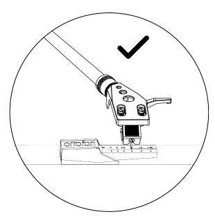
Adjust the counterweight until the stylus force gauge is in balance. Once the stylus is in balance, return the tonearm to its armrest. The anti-skate dial should be set to match the tracking force of the cartridge. Your factory-fitted cartridge has a tracking force of '2'.
