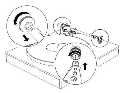
3. Release tonearm from rest and remove the stylus guard.
