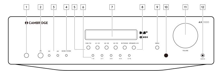
**1. POWER BUTTON** - Switches the unit between Standby mode (indicated by dim power LED) and On (indicated by bright power LED). Standby is a low power mode where the power consumption is less than 0.5 Watts. The unit can be left in Standby mode when not in use.
