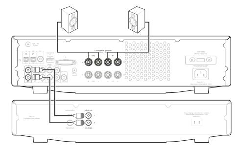
The diagram below shows the basic connection of the AXR100D to a turntable via the Phono input.
