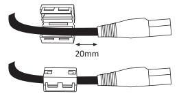
The hinged filter simply folds around the cable and will lock together once you firmly close the shaped channels around the cable. You should fit the filter at the end of the cable as shown. Allow a 20mm length of wire between the plug moulding and the filter. This will ensure optimum performance and allow good cable flexibility.
