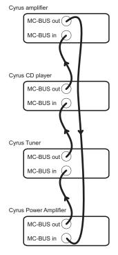
With MC-BUS connection established you can control the power function of the entire system from the front panel or remote control. Selecting 'CD' from the front panel will switch on the amplifier, the Cyrus power amplifier and a Cyrus CD player. When the amplifier is set to Standby, the entire system will also switch off.
