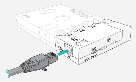
**NOTICE** Wi-Fi is disabled when an Ethernet cable is connected.
